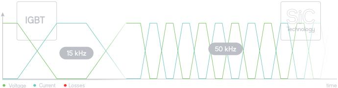
Transitioning to SiC technology results in an increased switching frequency of the converter, which translates into higher dynamics, faster transients and enhanced performance, making it the perfect candidate for EoL environments, R+D, Validation and Power Hardware in The Loop (PHiL) testing.
